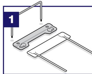
1 The U piece, pressure bar and adhesive base make up the 3 part clip.
